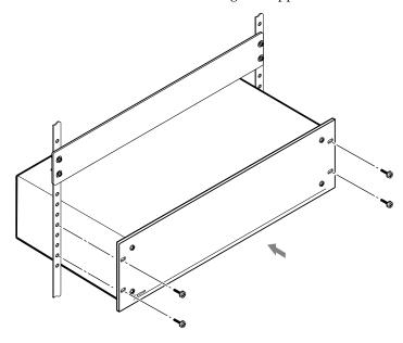
Figure 2-1 — Installing the switcher in a rack
